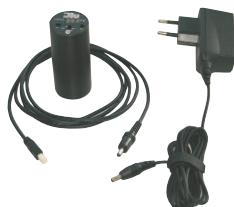
The readout unit „K01-Blue“ converts optical signals of devices with interface „IEC 62 056-21 (IEC 1107)“ in Bluetooth signals, which can be read by any PDA/PC with Bluetooth interface. Additionally it has a CS/CL-interface.
